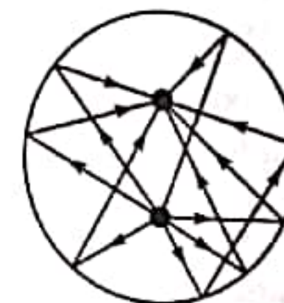
Fig. 2.13 : Cross-sectional view of the reflections in the cylindrical reflector
